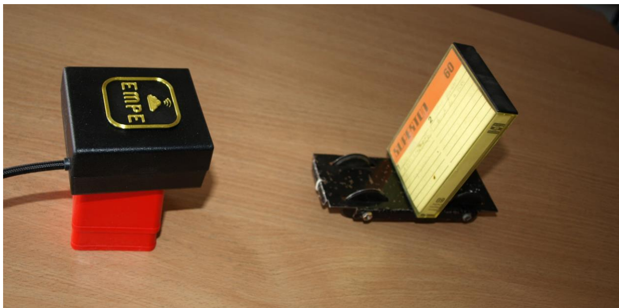
Fig. Example of using the EMPE sensor and a trolley with a flat wall to improve the precision of measuring changes in distance from the sensor.
