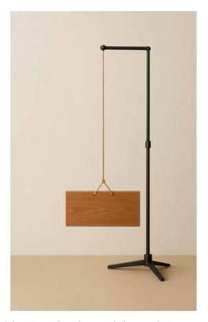
• Setting up the pendulum (e.g. a board suspended on a string).
