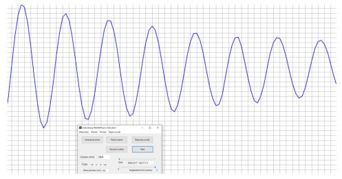
The recording frequency has a significant impact on the quality of the recorded data. We recommend setting the value to 100-150 [ms]. We recommend setting the sensor to measure distances of no less than 30 cm.
